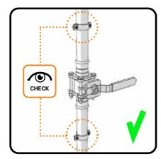
Valves must be supported by a pipe clip on both sides, with a maximum distance of 0.5m (20") between the valve and the pipe clips.
