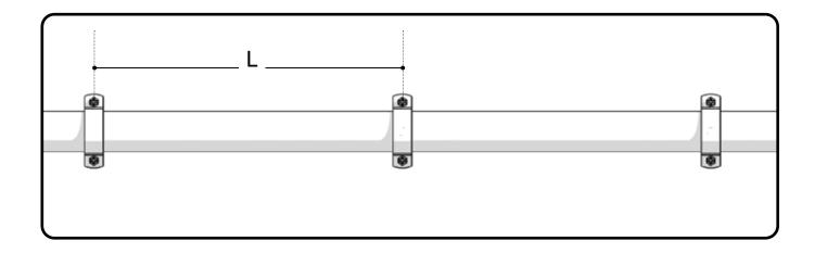
The maximum distance L between two pipe clips is given by the table below:
